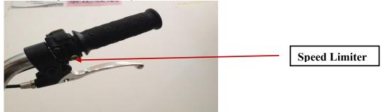
The speed limiter is located on the right side of the handlebar in the throttle housing, the speed will be limited
