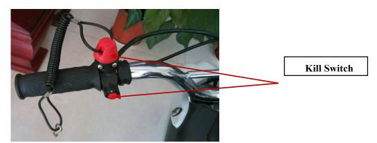
The emergency tether can be fastened to the rider in case there is an emergency. The engine will stop automatically when the rider pulls the tether.
